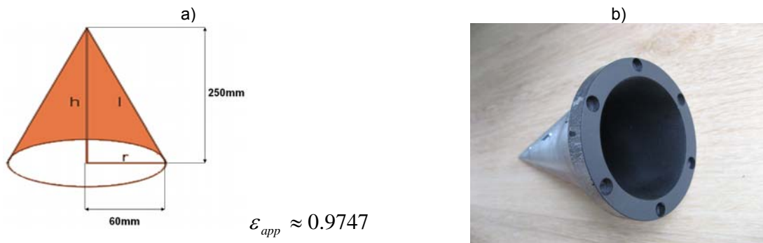
Fig. 1. Conical geometry and its computational emissivity a) and manufactured cone b)
